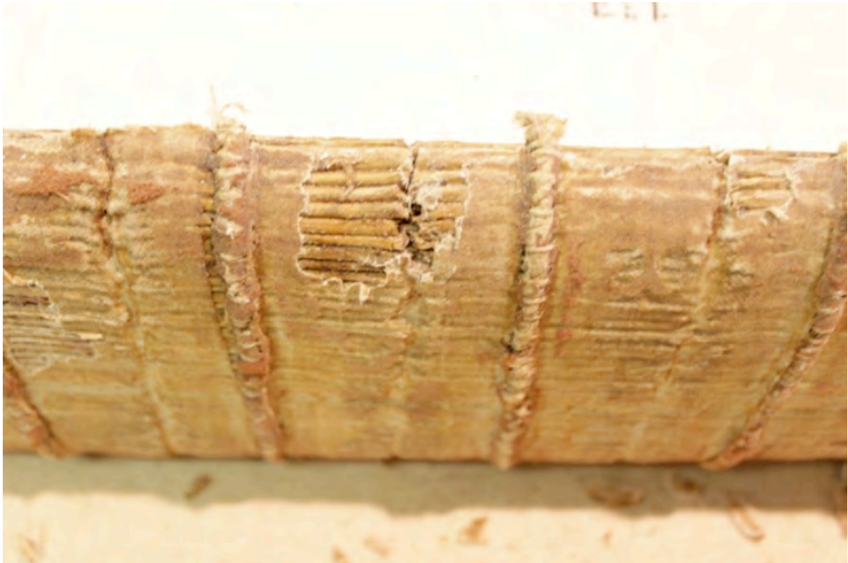
22-23. Spine with lining and thick layer of animal glue
